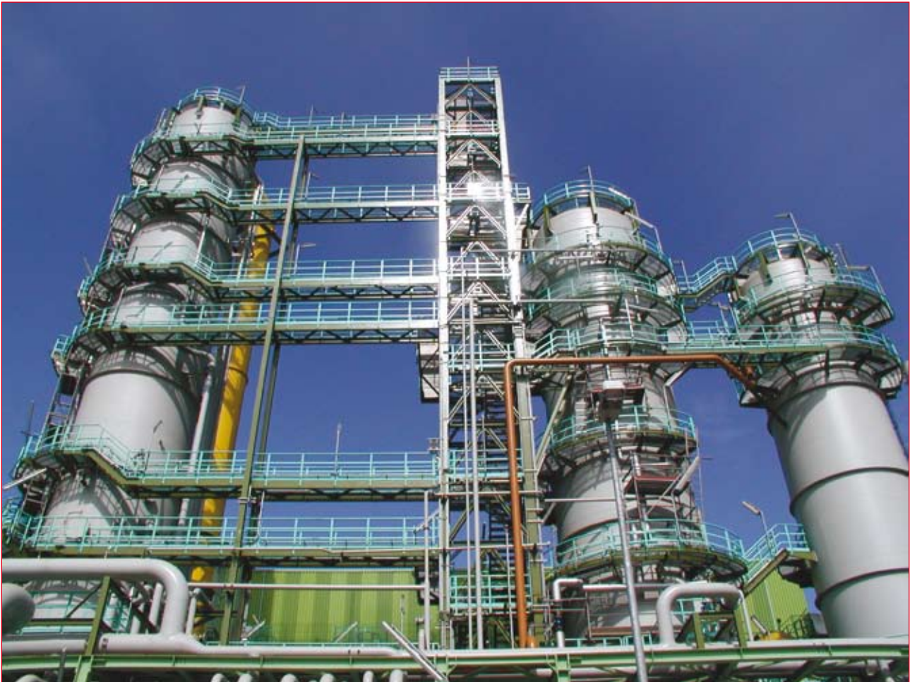
Typical large capacity syngas scrubbing vessel for removal of hydrogen sulphide, ammonia and BTX.
